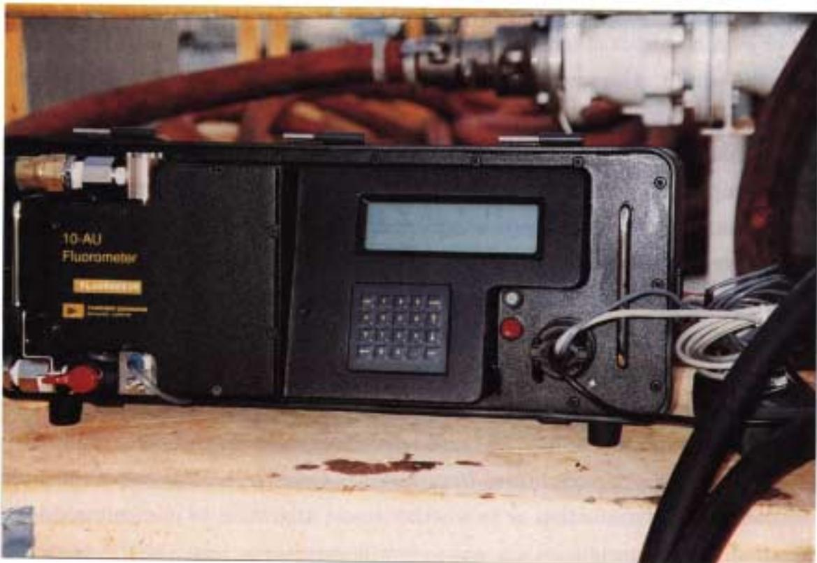
Figure 2. A Turner Designs® Model 10AU field filter fluorometer operating in the flow-through mode at Pearl Harbor Naval Base. The red valve is set horizontally to allow inflow of water from the bottom connector and discharge out the top connector.
