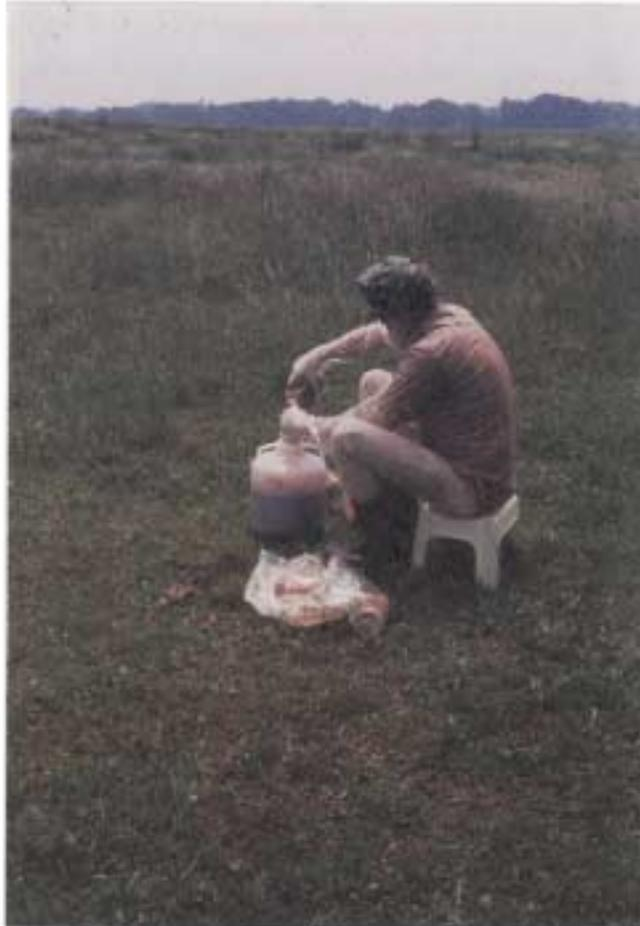
Figure 7. Mixing fluorescein powder dye with water in a 5 L carboy. Fluorescein is a brick-red color when a dry powder.
