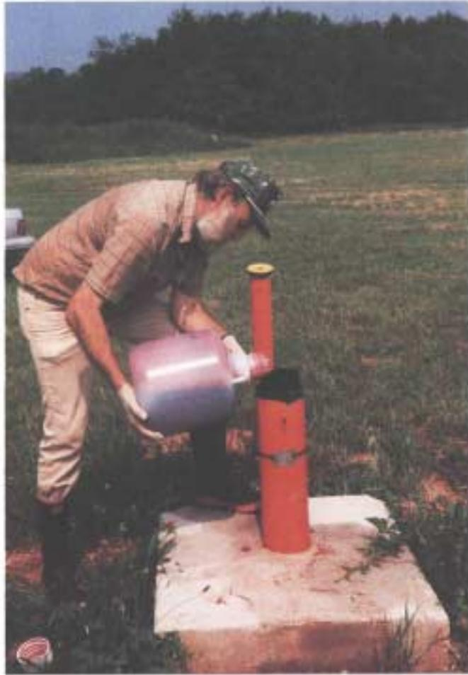
Figure 8. Injecting mixture of water and fluorescein dye into an injection well. Fluorescein has a dark red color when concentrated as shown here, but becomes a bright fluorescent green when diluted.
