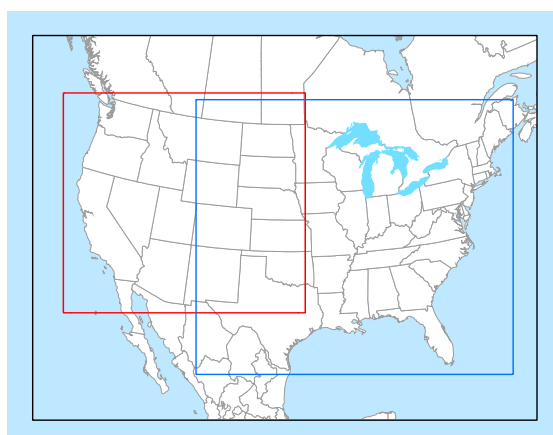
Figure 2-43. CMAQ modeling domains for the OAQPS risk and exposure assessments: 36 km outer parent domain in black; 12 km western U.S. (WUS) domain in red; 12 km eastern U.S. (EUS) domain in blue.
