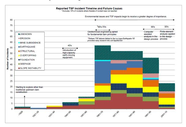
Figure 1. Tailings Failure Statistics<sup>1</sup>
