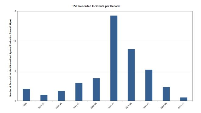
Figure 2. TSF Failures/Mtpa tailings production<sup>2</sup>
