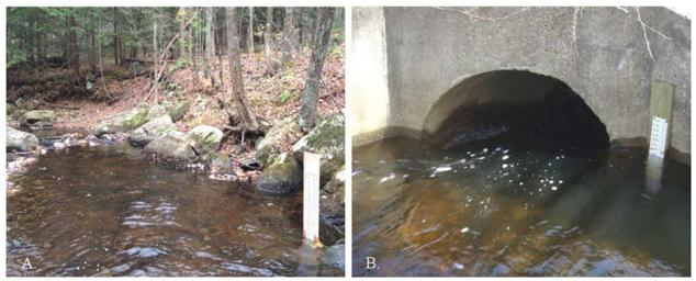
Figure 17. Examples of controls downstream of staff gages include A. riffle and B. culvert.
