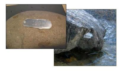
Figure 12. Metal forestry tags can be attached to the downstream side of large rocks to monument sites and air in relocation of sensors (Isaak et al. 2013).
