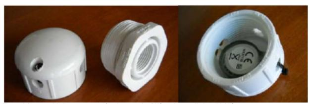
Figure 4. Unassembled components of an inexpensive PVC canister radiation shield for water temperature sensors (described in more detail in Isaak et al. 2013).
