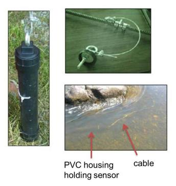
Figure 10. Photos of a rebar installation (from Mauger 2008).
