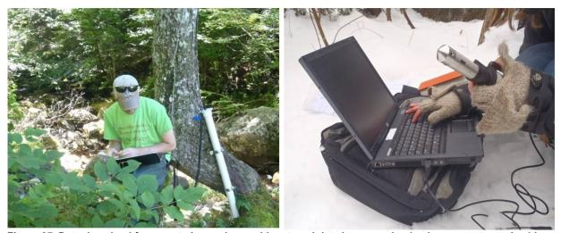
Figure 27. Data download from vented transducer with external data logger on land using computer and cable (left) and non-vented transducer with internal data logger using computer and data shuttle (right).
