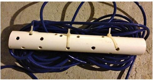
Figure 15. Example of a protective housing made of PVC pipe. This one is for a vented pressure transducer, which is secured inside the pipe with zip ties. If vandalism is a concern, the PVC can be painted to make it less visible.
