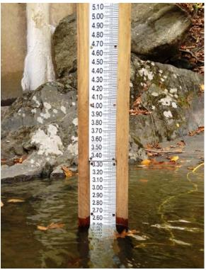
Figure 14. Example of a USGS style staff gage (Type A) marked in 0.02 foot increments.
