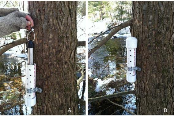
Figure 24. Barometric pressure sensor installation for a non-vented transducer A. without the PVC cap on top and B. with the PVC cap.
