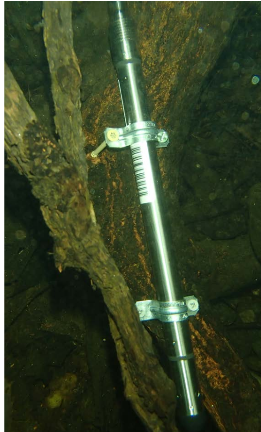
Figure 19. Some transducers come in a protective metal case and do not need to be encased in an additional housing.
