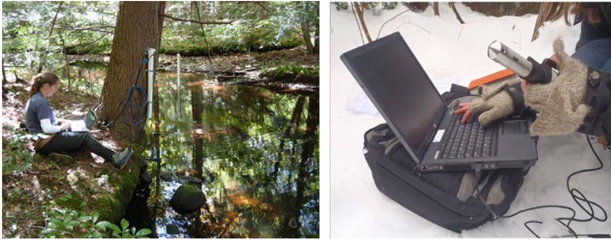
Figure 31. Data download from vented transducer with external data logger on land using computer and cable (left) and non-vented transducer with internal data logger using computer and data shuttle (right).
