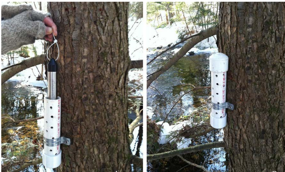
Figure 28. Barometric pressure sensor installation for a non-vented transducer, A. without the PVC cap and B. with the PVC cap. Holes should be drilled into the bottom cup of the PVC housing. This prevents condensation and laterally blown rain and snow from filling the cup to a depth sufficient to inundate the ports through which the barometric pressure is compensated. Another option is to deploy the barometric pressure sensor upside down, so that the port tip is on top.
