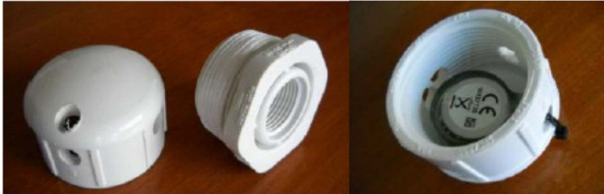
Figure 4. Unassembled components of an inexpensive PVC canister radiation shield for water temperature sensors (described in more detail in Isaak et al. 2013).
