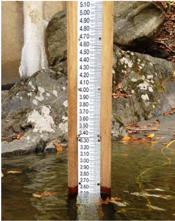
Figure 17. Example of a USGS style staff gage (Type A) marked in 0.02-foot increments.
