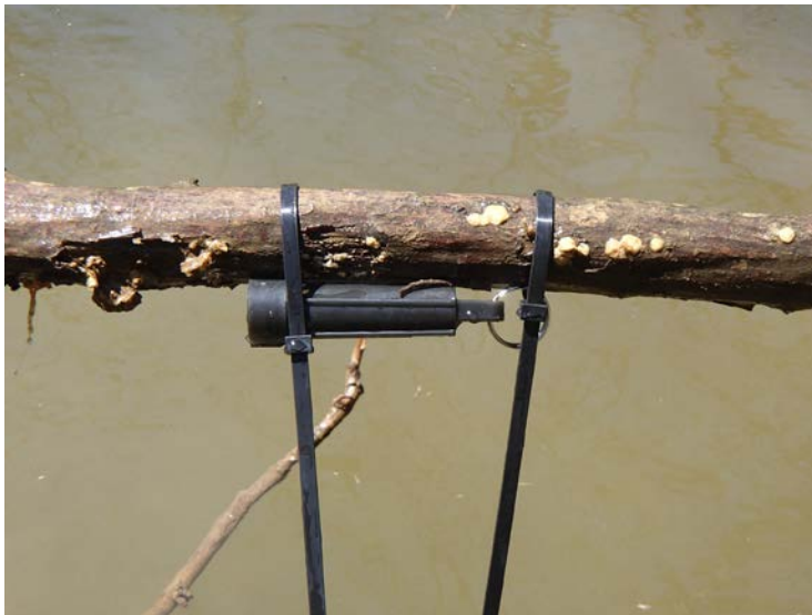
Figure 10. If conditions permit, attach sensors in two places, using heavy-duty (e.g., 120-lb tensile strength) cable ties. This picture was provided by MDDNR Monitoring and Non-Tidal Assessment.
