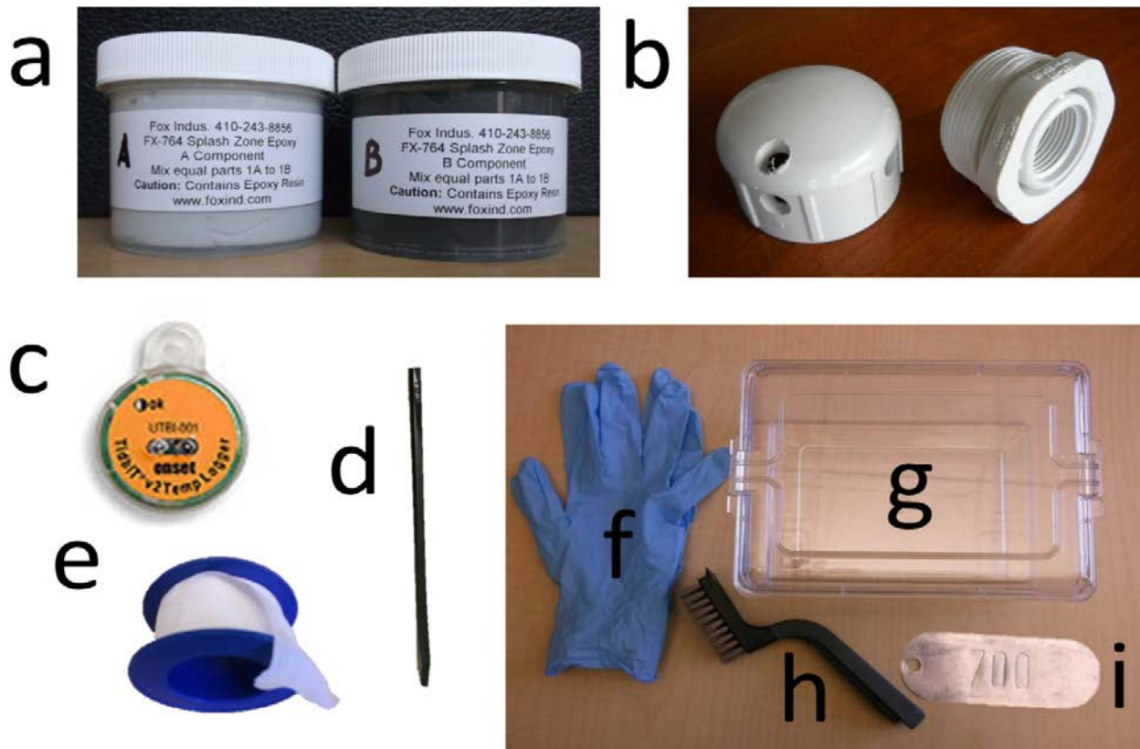
Figure 9. Equipment needed to permanently install temperature sensors in streams using underwater epoxy. The equipment includes: (a) two-part FX-764 epoxy from Fox Industries, (b) PVC solar shield, (c) temperature sensor, (d) cable ties, (e) plumber's tape, (f) rubber gloves, (g) plastic viewing box, (h) wire brush, and (i) metal forestry tree tag (Isaak and Horan 2013).
