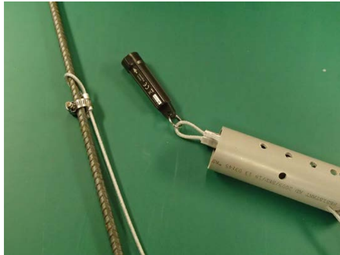
Figure 12. Example of how a cable and rebar installation is configured for large streams in Maryland. During the field installation, the cable is tightened so that the sensor sits within the PVC housing. Heavy-duty cable ties are then run through two of the side holes in the PVC housing to secure the sensor to the side of the PVC. This picture was provided by MDDNR Monitoring and Non-Tidal Assessment.
