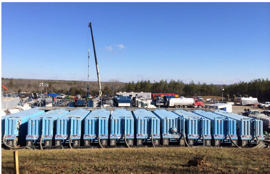
Figure 2-10. Water tanks (blue, foreground) lined up for hydraulic fracturing at a well site in central Arkansas.
