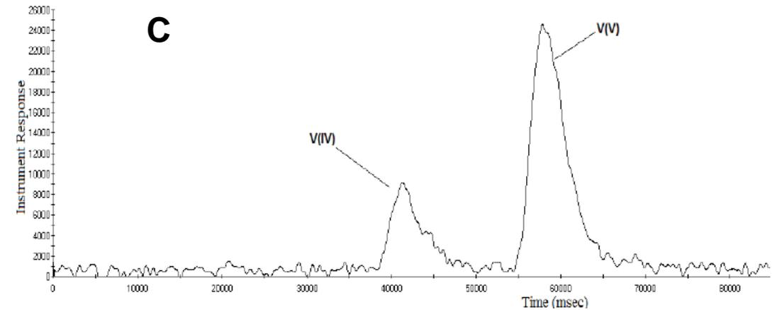
Plasma matrix standard of V<sup>+5</sup> showing conversion of V<sup>+5</sup> to V<sup>+4</sup>
