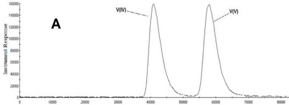
Solvent standards showing stability and separation of V<sup>+4</sup> and V<sup>+5</sup>
